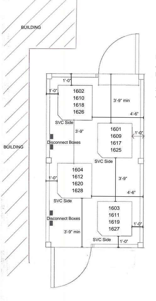
Each Owner has an HVAC unit location that is specific to that Address Number based on the proximity to the access lines. HVAC unit size based on standard 36" square. Placement guidelines will be strictly enforced.
